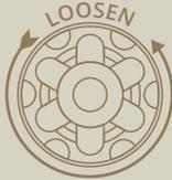
To remove the ADAPT Module, first remove the muzzle cap from the end of the Module using the supplied tool. This is accomplished by inserting the grooves of the tool into the corresponding grooves in the muzzle cap and rotating the tool counter-clockwise until removed.
