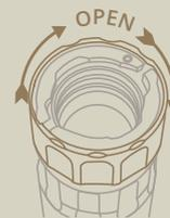
2. Hold the suppressor by the main body and thread suppressor onto the muzzle device until it is fully seated. Do not thread on using the locking collar.
