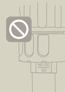
INCORRECT installation shown via NO-GO gauge
